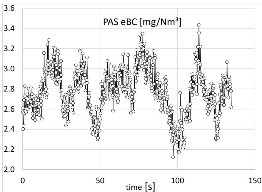
**Figure 5: Exemplary variation of eBC emission over time during one integral PAS measurement**
