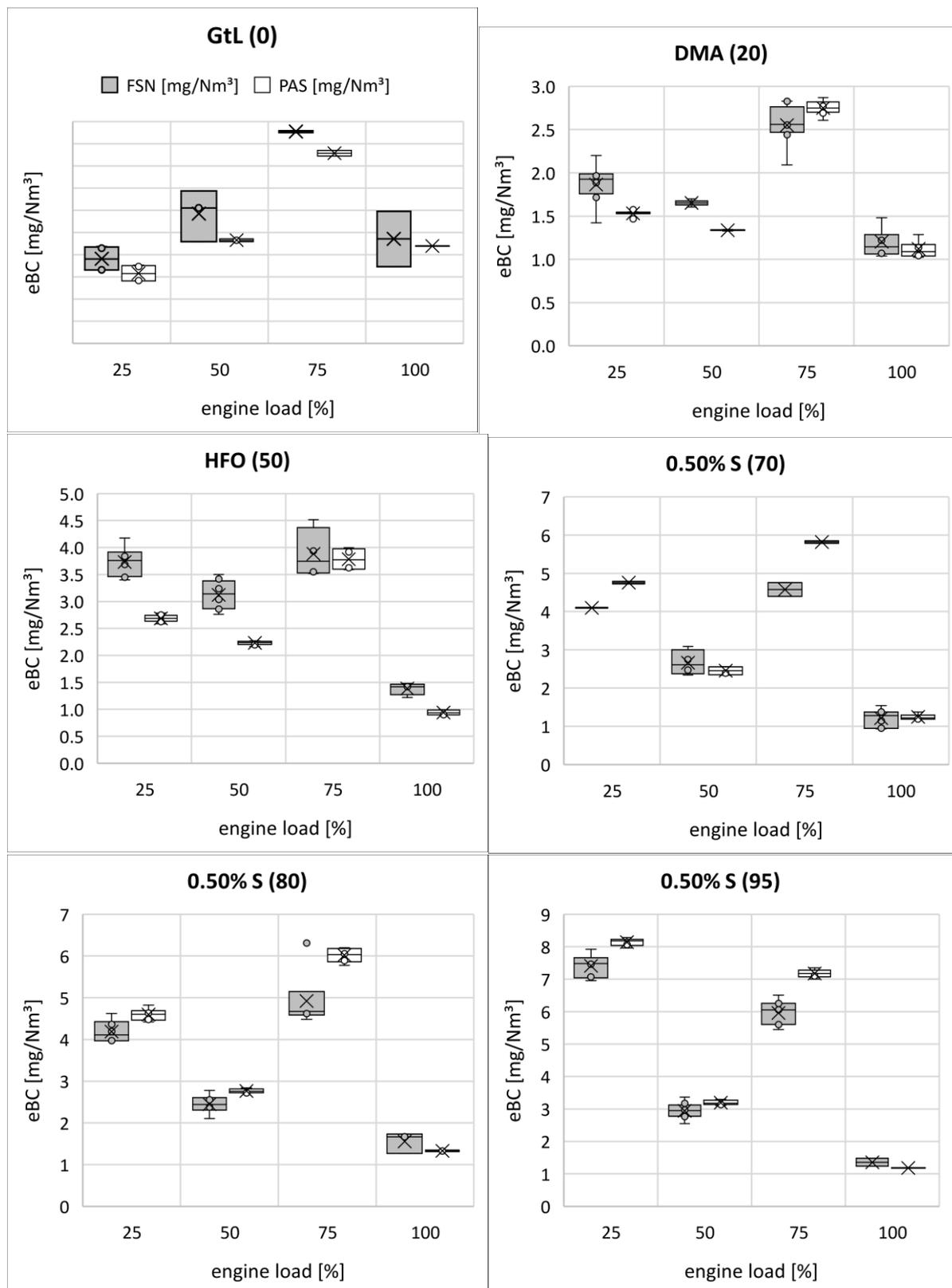
**Figure 2: Box and whisker plots for eBC emissions in mg/Nm³ (FSN and PAS) versus engine loads for each tested fuel (GtL, DMA, HFO, and the three 0.50% sulphur fuels; in brackets the aromatic content). The legend can be found in the box plot for GtL. Note: The y-scales vary, due to the different concentration ranges.**
