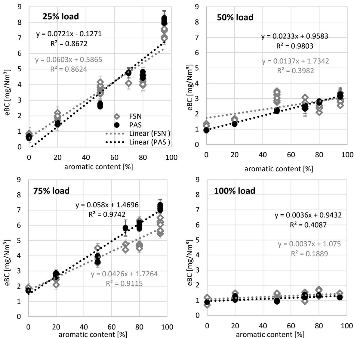
**Figure 3: eBC emissions for 25, 50, 75 and 100% engine loads in relation to fuel aromatic content (the legend for FSN and PAS identification is in the diagram for 25% load)**
