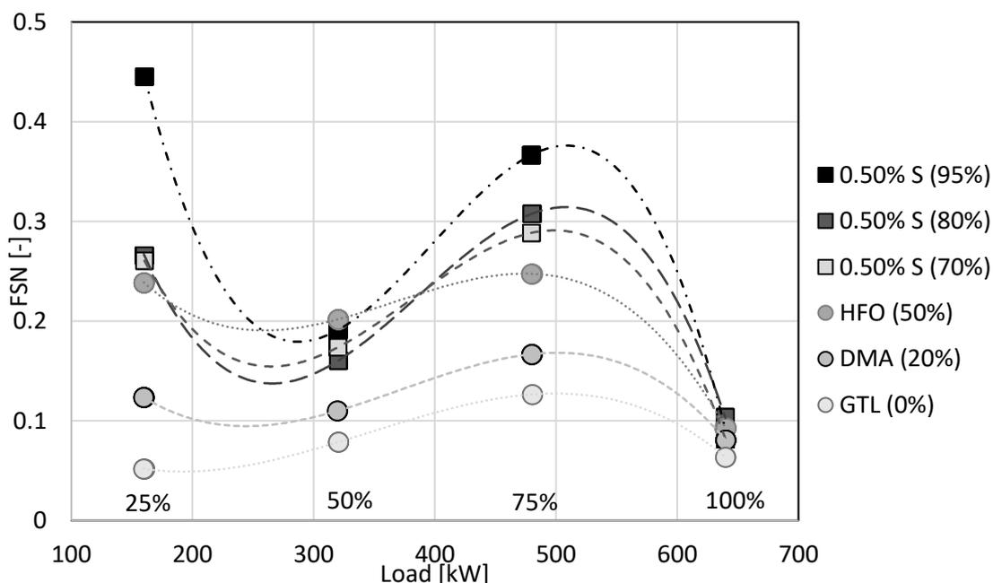
**Figure 1: FSN values versus power output [kW] / engine load [%]**
